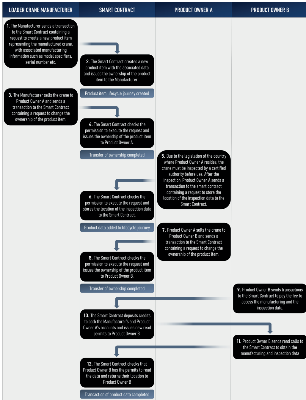
Figure 1 Participation protocol for blockchain-based deployment of product-centric information management over the life-cycle of a loader crane
